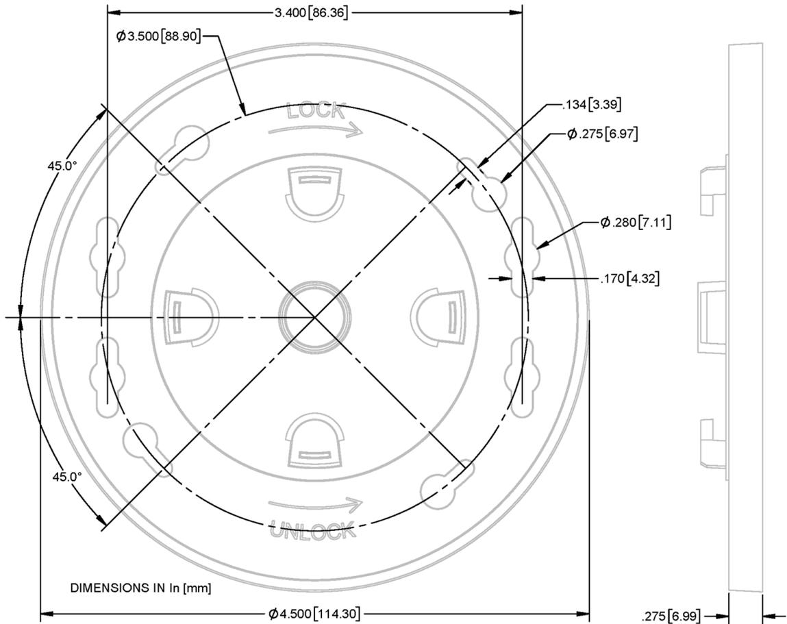
3. Drill holes for the screws and insert anchors.
